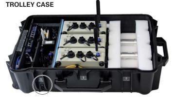
Full set of three units assembled for easy campaign deployment. Embedded power supply from main.
